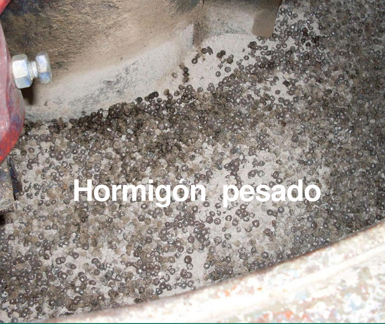
A close-up photograph of heavy concrete aggregate, showing numerous dark, spherical particles of varying sizes embedded in a light-colored matrix. A metal bolt is visible on the left side of the frame.
